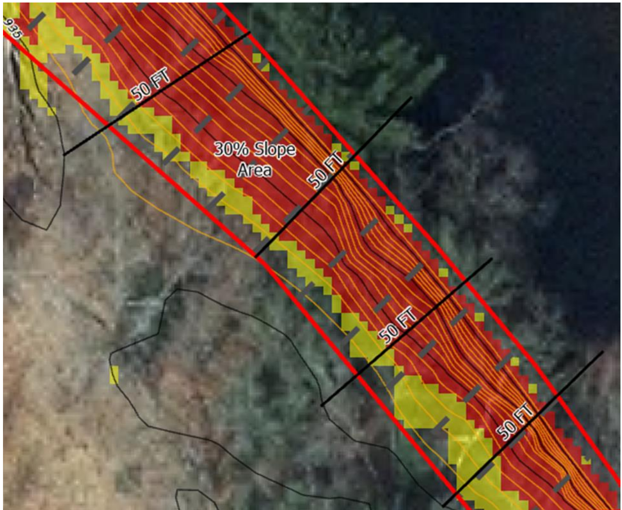
Figure 3 – Slopes with a Horizontal Distance of less than 50': The elevation change depicted by the black lines drawn perpendicular to the contour lines represent the 50ft horizontal distance used to calculate slope as a percentage. Areas that have slope over 30% are shown by the dashed hatching within the red outline. Even though the total horizontal distance of the digitally created slope color is not 50 feet long, it still qualifies as a steep slope, because the slope measured within 50' horizontal increments is greater than 30%.
