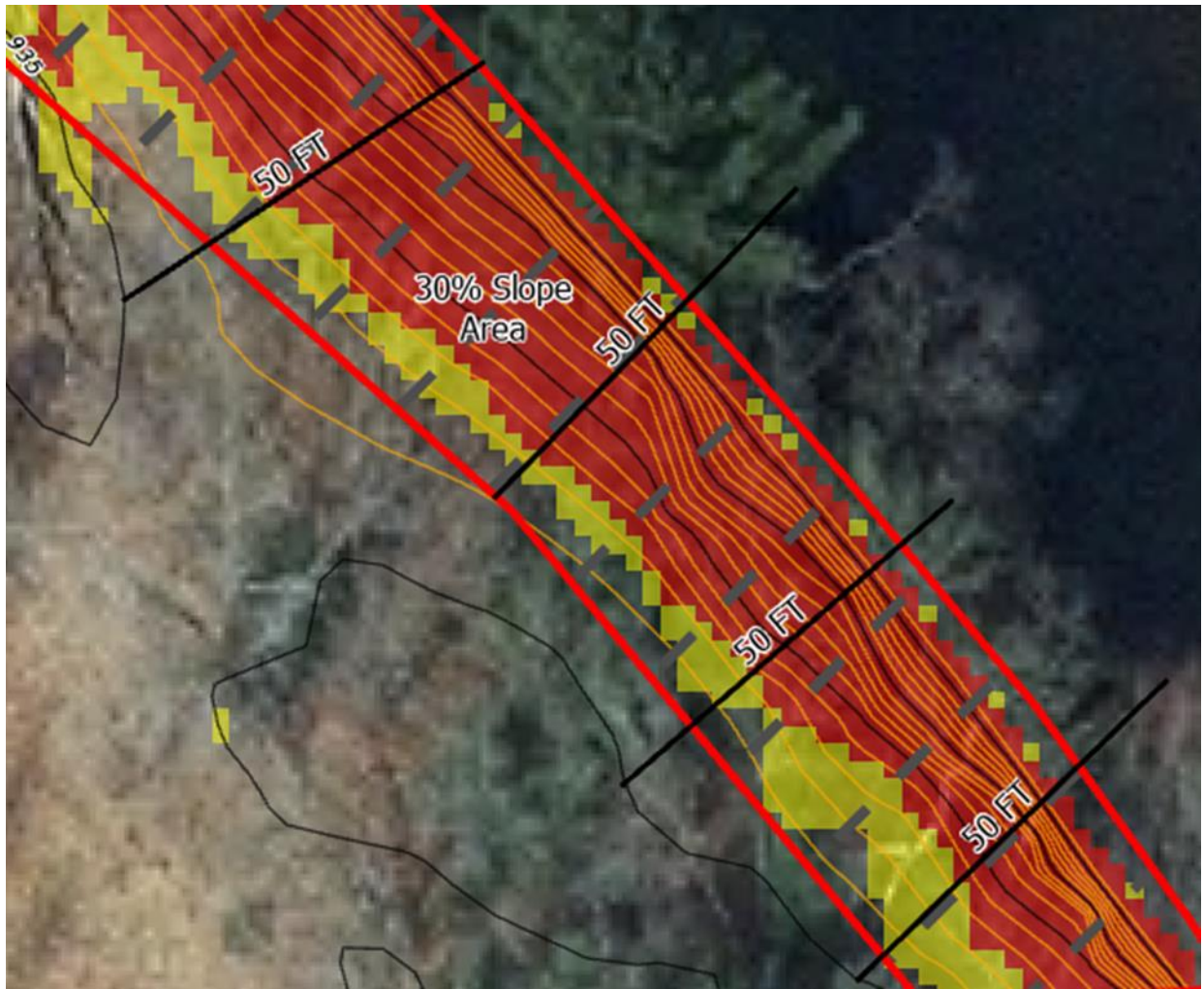
Figure 3 – Slopes with a Horizontal Distance of less than 50': The elevation change depicted by the black lines drawn perpendicular to the contour lines represent the 50ft horizontal distance used to calculate slope as a percentage. Areas that have slope over 30% are shown by the dashed hatching within the red outline. Even though the total horizontal distance of the digitally created slope color is not 50 feet long, it still qualifies as a steep slope, because the slope measured within 50' horizontal increments is greater than 30%.
