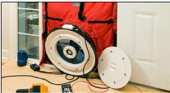
Blower door test being performed.
