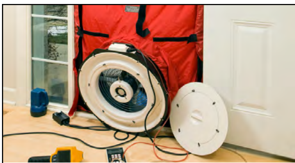
Blower door test being performed.
