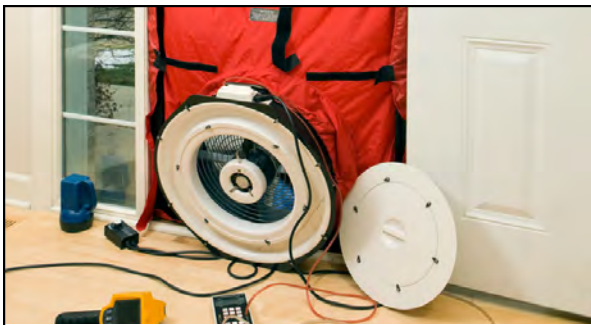
Blower door test being performed.
