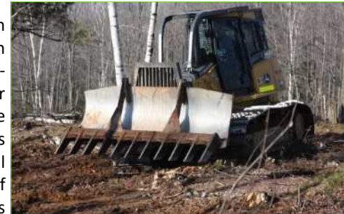
Dozer conducting mechanical soil scarification in recently harvested birch stand
