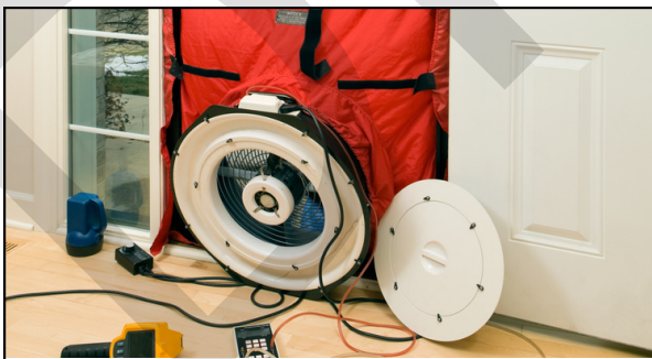
Blower door test being performed.
