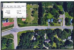
It should be noted that changes to a regulatory speed limit should not be used to correct spot safety issues. Instead, improvements to the physical environment should be considered. In this case, clearing of the intersection sight distance triangle should be investigated.
