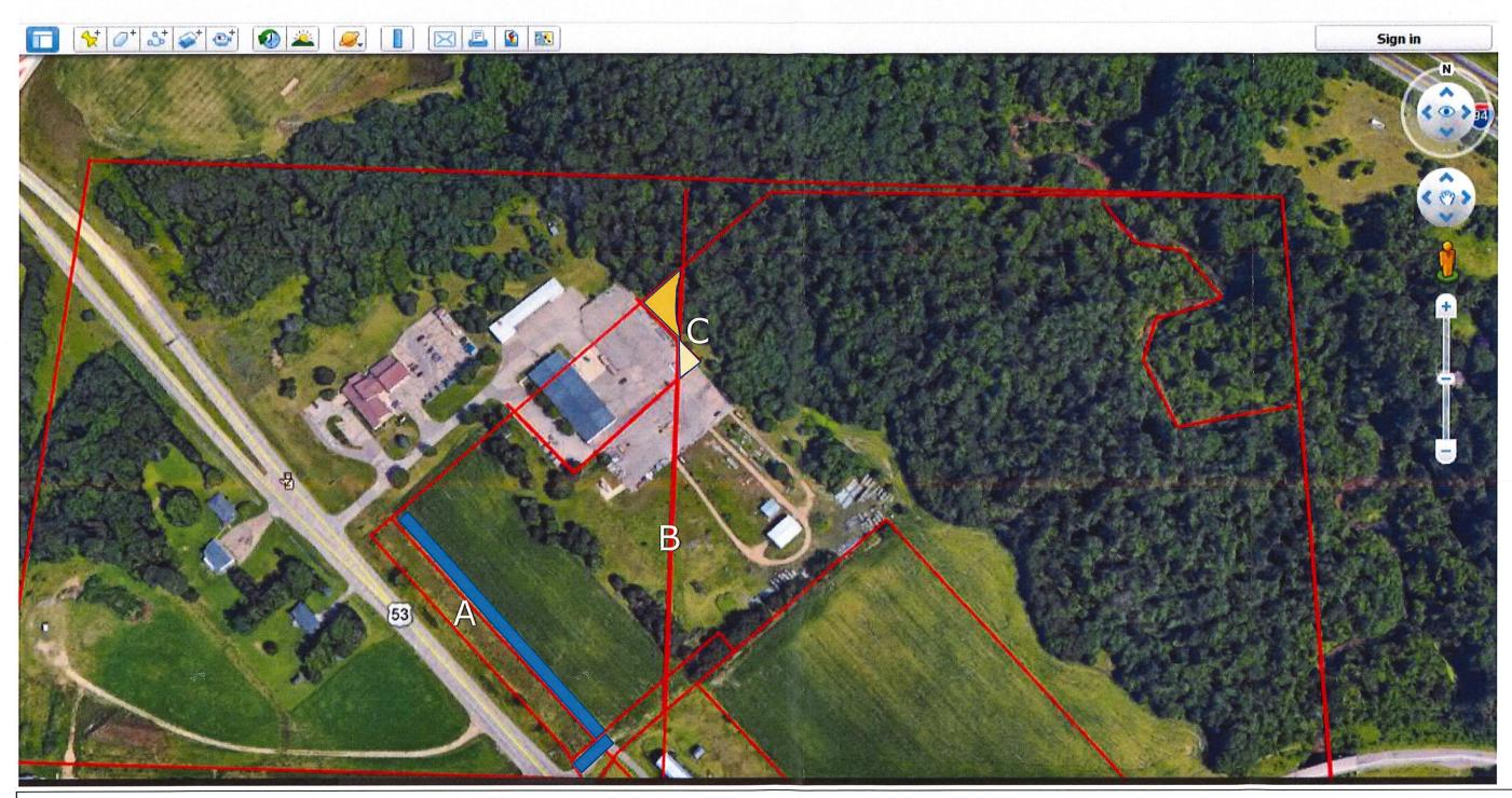
A – Have confirmed the 'inner' line is the highway ROW line (120' from reference line).
