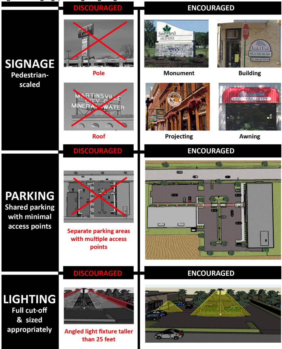
Figure 2.4: Signage, Parking & Lighting
